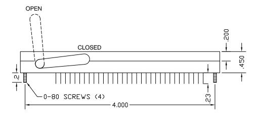
This series is designed for long in-line packages that are wider than two rows, with either square or staggered device lead patterns.
